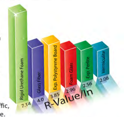
Comparison & Properties of different insulation materials available in Pakistan.
